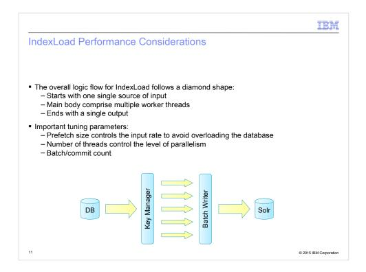
Since the processing flow in Index Load is comparable to a diamond shape, with a single reader in one end, a single writer in the other and a number of parallel worker threads in the middle, three important settings have an impact on overall performance:
