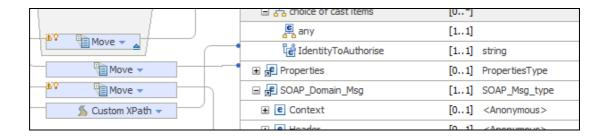
Observe that the Custom XPath transform has been defined with the following transform (click on the transform to bring its properties into view).
