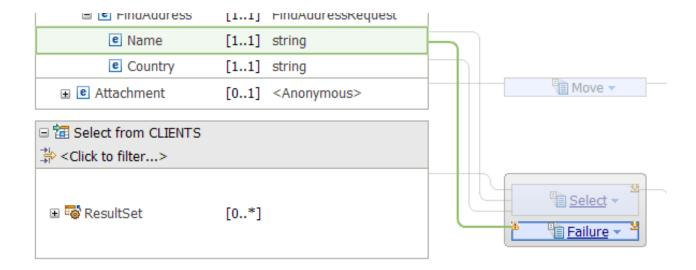
3. Connect the message assembly element **Country** to the **Failure** transform. The following figure shows the element **Country** connected to the **Failure** transform:
