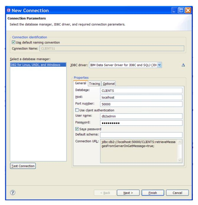
5. In the New Connection - Connection Parameters, click **Finish**. The **CLIENTS1** connection is created.
