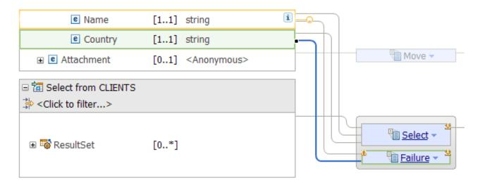
4. Connect the Failure transform to the output element Fault.
