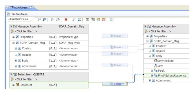
3. Set the cardinality of the **Input array indexes** to 1 in the **Select** transform properties view to indicate that you only wish to work with the first row of the result set returned by the database.
