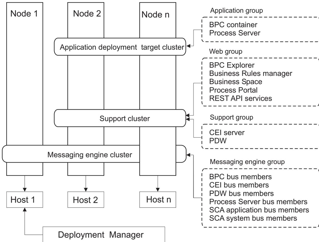
Figure 5. Remote Messaging and Remote Support topology pattern
