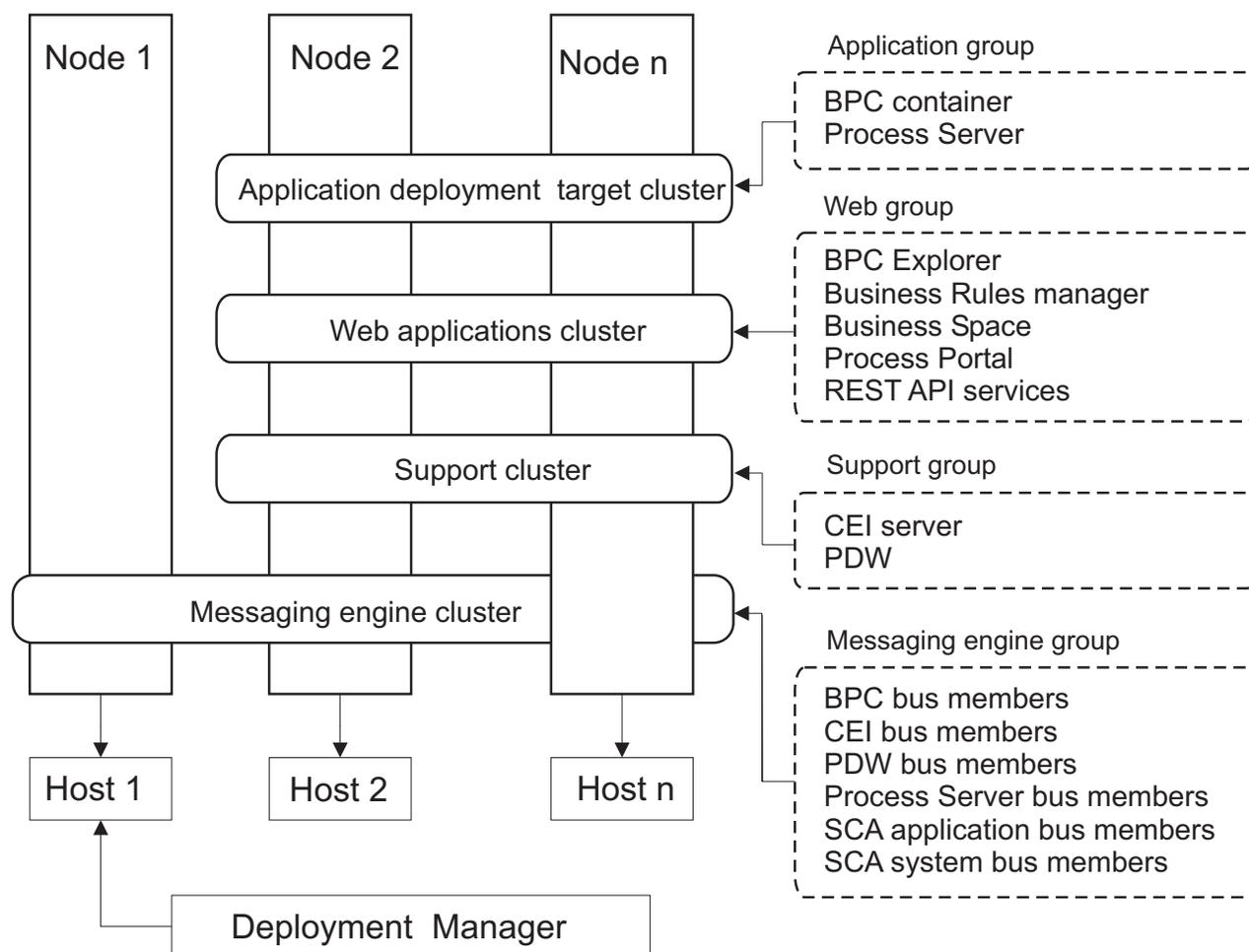
Figure 7. Remote Messaging, Support and Web topology pattern
