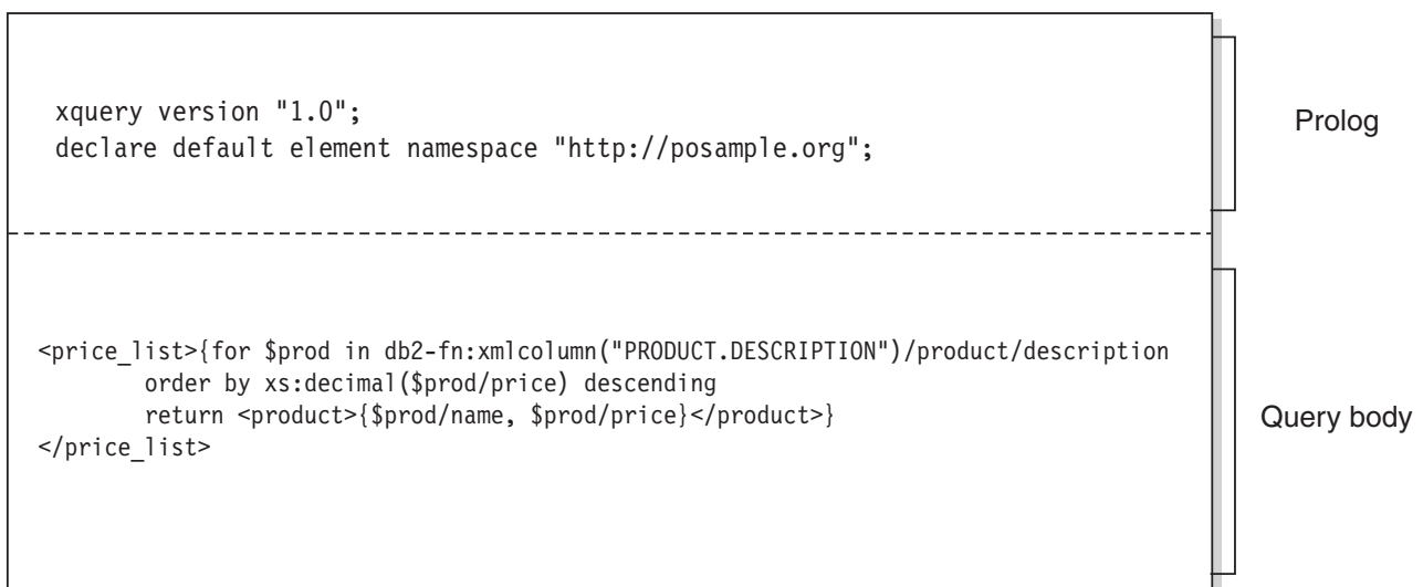
Figure 4. Structure of a typical query in XQuery
