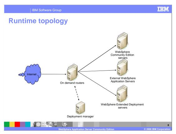
As this diagram shows, the on demand router is capable of routing requests, not only to WebSphere Application Server managed servers, but also to WebSphere Community Edition servers, external WebSphere Application server, and other HTTP endpoints. The on demand router retrieves information about servers and applications that are active in the cell, allowing it to accurately route HTTP requests to those application servers which are currently running.
