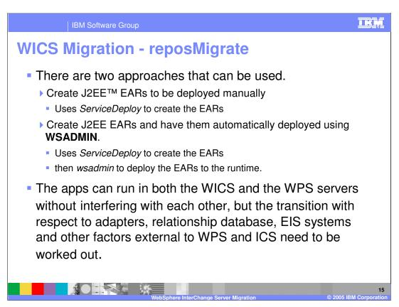
**reposMigrate** is the WPS command line utility for converting the WICS artifacts to WPS/SCA artifacts. reposMigrate can also invoke the ServiceDeploy utility to package the WPS/SCA artifacts into jars and EARs.
