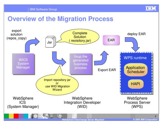
From a high level perspective, the migration process consists of the following steps: export from the source system, import to the target system, edit, resolve errors and tune the migrated artifacts for BPEL / SCA and deploy the application to the WPS V6 runtime.
