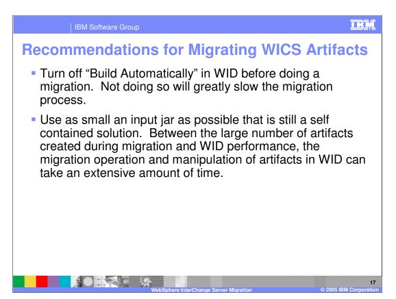
The migration process creates many new artifacts and if the autobuild feature is on, a build will be started before all the artifacts have been created. As new artifacts are created, new builds are also started. The result is a degradation in the overall build performance.
