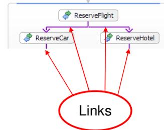
Links and link conditions are associated with flow activities and can include conditional logic to determine if processing should proceed on a particular path. This has been enhanced in WebSphere Process Server V6.0 to include support for XPath. Conditions can also be evaluated using Java programming, an IBM extension, or a value of true or false can be hard coded into the link. Parallel execution can be performed during a long-running business process if multiple conditions evaluate to true.
