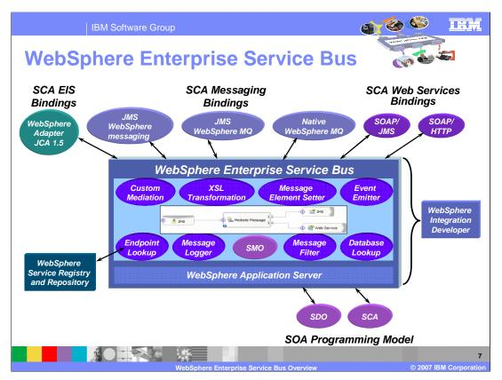
The SCA Import and Export binding types have now been added to the picture. These define the possible transport protocols that can be used with the WebSphere Enterprise Service Bus for receiving service requests and for making calls to service providers. The SCA bindings used with WebSphere Enterprise Service Bus are not unique but are the same SCA binding types available with WebSphere Process Server.
