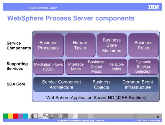
This slide expands on the previous slide to show the additional components that WebSphere Process Server introduces in addition to what WebSphere Enterprise Service Bus provides. As you can see, all the components of WebSphere Enterprise Service Bus are included in the WebSphere Process Server.
