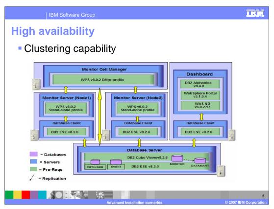
This chart depicts an installation scenario for clustering. In this specific case one machine is the cell manager with two separate machines in the cell containing Monitor Servers. There is another machine for the Dashboard Server, and another machine containing the Database server. You can install as many Monitor Servers into the Cell as you have licenses.
