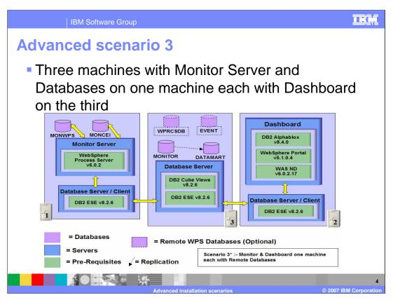
This chart depicts an installation scenario with three machines, one for the Monitor Server, one for the Dashboard Server, and a third machine with the Database server. This might be the preferred topology if you require a separate database server.
