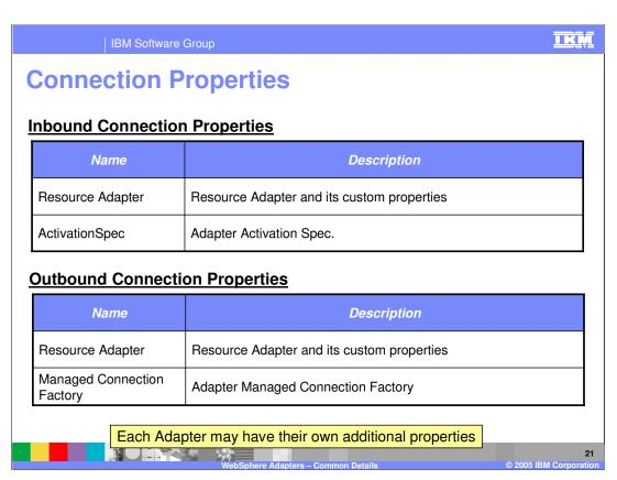
As indicated in the previous page, the properties for the Inbound request are in the Resource Adapter and the ActivationSpec, whereas the properties for the Outbound request are in the Resource Adapter and the Managed Connection Factory.
