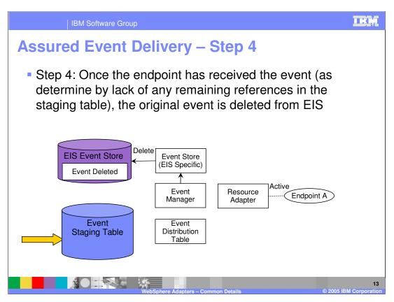
In the last step 4, once the endpoint has received the event, the original event in the EIS Event store is marked for deletion. The event is now considered processed end to end.
