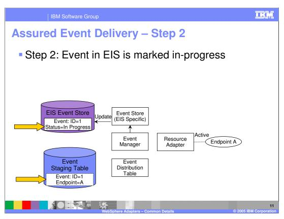
In step 2, the event is saved in the Event staging table within the adapter along with the event ID, the endpoint that is the registered listener of the event.
