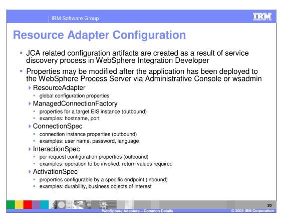
When the developer uses the Enterprise Service Discovery wizards to create the outbound or inbound request to and from backend EIS, the JCA properties for the Resource Adapter, Managed Connection Factory for outbound request and ActivationSpec for inbound request are already created based on the input to the service discovery wizard.
