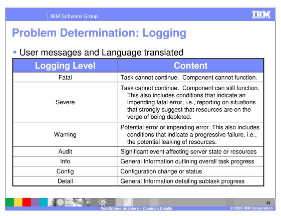
The different logging levels are specified on this page. These messages are translated and they appear in the WebSphere Process Server System out log files.
