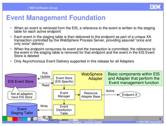
This diagram shows the different components that enable the event management framework to handle incoming events. This is provided by the Adapter foundation classes for all the adapters to exploit.
