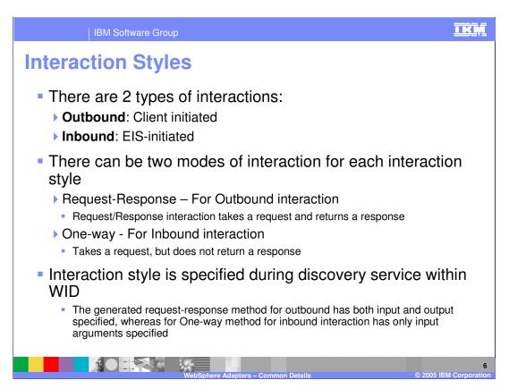
A outbound request or interaction is initiated by a client. The client could be a SCA component within the same module or some other module, or could be some external client like a JSP.
