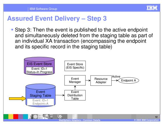
In step 3, the event is published to the active endpoint and deleted from the staging table. The two actions might be part of an XA transaction if the endpoint supports transaction. The delivery of the event to the endpoint indicates the end of the transaction.
