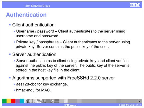
If server authentication is disabled, the client will trust any server and will connect to it if other connection parameters are correct. It is recommended to always enable server authentication.
