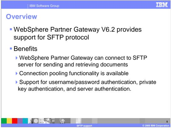
SFTP stands for Secure File Transfer Protocol. It is different from FTP (File Transfer Protocol). It provides the functionality of message integrity, confidentiality, and authentication. It also provides multiplexing of documents using different channels. In WebSphere Partner Gateway, there is an additional benefit of connection pooling, as the SFTP functionality is provided using J2C resource adapter.
