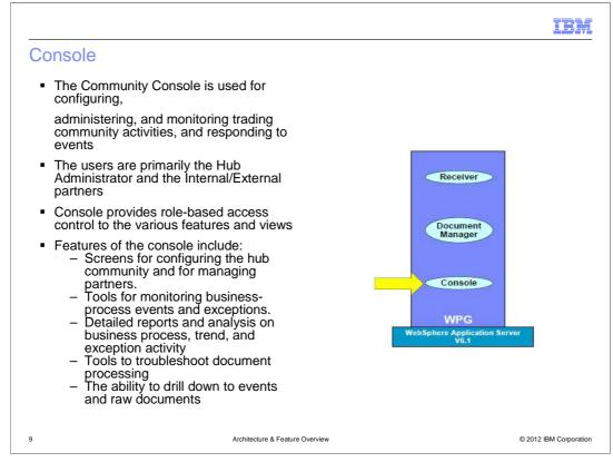
The Console is the web interface for the Community Operator, Internal Partner, or the External Partner to configure. It is also used to administer and monitor the trading activities. Based on the type of user logged in to the console, appropriate functions are exposed based on the user's role. The console also provides an interface to a set of tools that allow you to view the documents that have flowed through the hub and provides troubleshooting for failed documents
