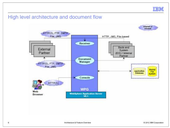
The slide shows the high level architecture and high-level view of the document flow through the WebSphere Partner Gateway hub components. This architecture is similar to V6.0. There are three major WebSphere Partner Gateway components, namely the Receiver, Document Manager and Console.
