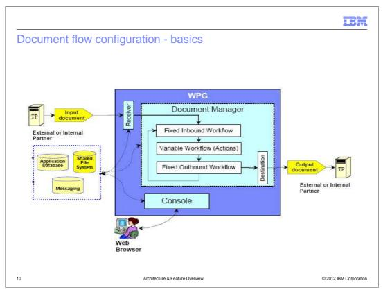
This graphic provides more detail about the basic flow within WebSphere Partner Gateway components, especially the Document Manager. There are three different workflows for every document passing through the document manager. First, the fixed inbound workflow is used for a fixed set of work actions that apply to all incoming documents.
