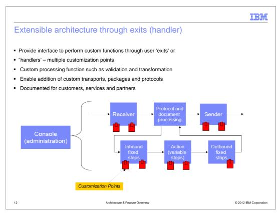
WebSphere Partner Gateway provides a mechanism for adding custom functions called exits or handlers at different stages of document processing. It includes support for many pre-defined packages, protocols and document types. With the pluggable extensibility of the architecture, new custom packages, protocols or document types can be added by the hub administrator.
