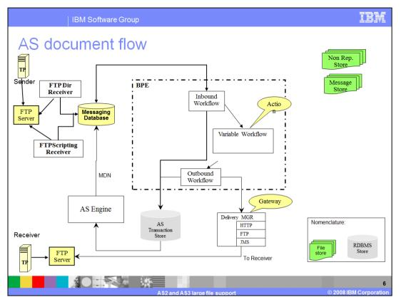
This slide describes the sample workflow inside WebSphere Partner Gateway. Although the workflow is specific to AS3, AS1 and AS2 goes through the same steps, the difference is only in the transport protocol.
