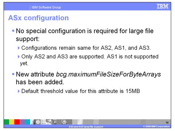
There are no changes to the Configuration and it remains the same as the previous release for AS1, AS2, and AS3. A new attribute "bcg.maximumFileSizeForByteArrays" has been added. The default value for this attribute is 15MB.
