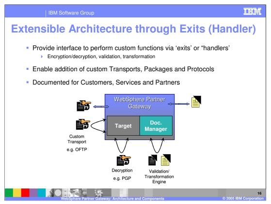
WebSphere Partner Gateway provides a mechanism for adding custom functions called exits or handlers at different stages of document processing. This support is used to expand capabilities such as the addition of the new native EDI functionality. The functionality of the exits or handlers are carried forward from WebSphere Business Integration Connect v4.2 release. Listed below are some examples of architecture extension through the use of exits and handlers.
