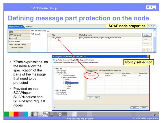
This slide shows how the properties of the SOAP Nodes are used to specify security on parts of the SOAP message.
