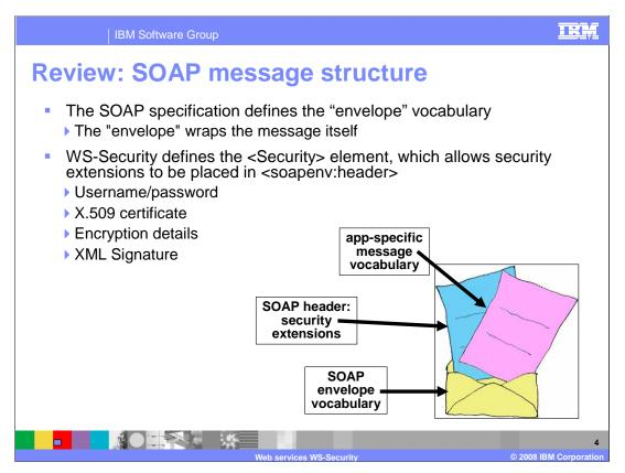
A SOAP message consists of an envelope, which contains the whole message. Within the envelope is the actual message, which consists of header information and a SOAP body. The body is the real payload, the message which an application program will typically need to access.
