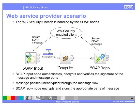
This slide shows the scenario where the message flow represents the Web service. A Web service client invokes the message flow by sending it a SOAP message. In this case, the SOAP message is secured using WS-Security.
