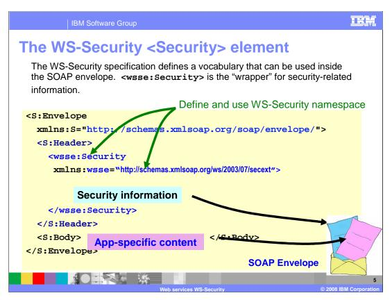
The example shows a SOAP message with a skeleton showing where WS-Security should be placed.
