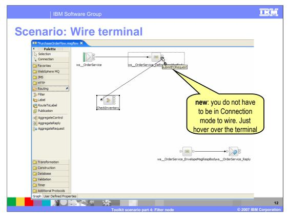
Wire the submit terminal (submit for request) of the Subflow node to the input of the added Filter node named CheckInventory. New in V6.0.2, you do not have to be in Connection mode to wire, just hover over the terminal. This concludes part 4 of the WebSphere Message Broker V6.0.2 Toolkit scenario.
