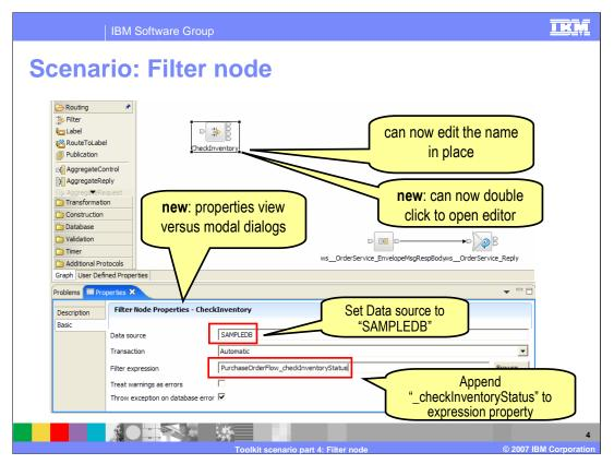
Drag and drop a Filter node to the Purchase Order message flow previously generated and name the node in place. In the Properties view specify the database, SAMPLEDB, as the Data source and set the Filter expression to checkInventoryStatus.
