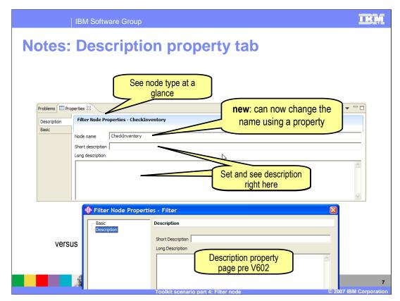
The node type is displayed at the top of the Properties view, and the name of a node can be changed in the Description property tab.
