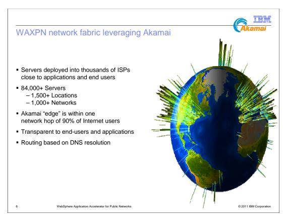
The WAXPN Network fabric consists of more than 80,000 servers in 1500 locations worldwide. A WAXPN edge server is within one network hop of 90% of Internet users. This service uses DNS resolution To route requests to edge servers and is therefore transparent to end users.
