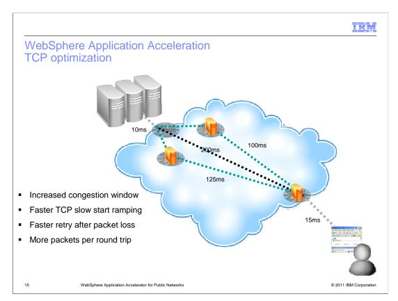
The Akamai overlay also performs transport TCP optimizations to improve latency and throughput. Some examples are, increased congestion window, faster TCP slow start ramping and faster retry after packet loss.
