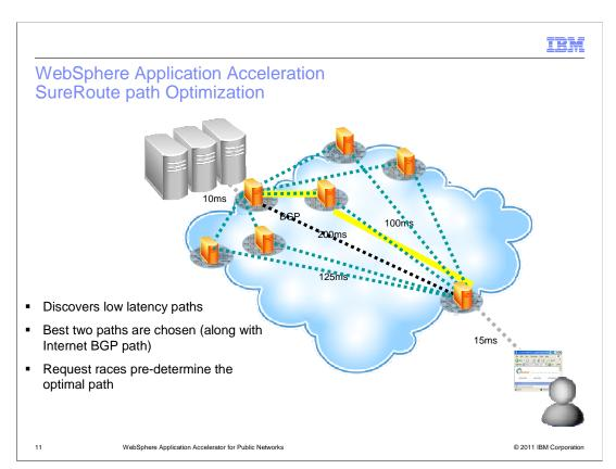
Sure Route path optimization uses parallel requests on disjoint paths to determine and cache the fastest or lowest latency paths across the Internet. The redundant disjoint paths can also be used for fail-over purposes.
