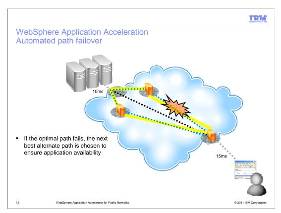
If the optimal path fails, the next best alternative disjoint path is chosen to ensure application availability. Alternative paths are cached and thus convergence time is fast. For example, in this picture, the two best paths are highlighted in yellow. Once the top most path fails, the bottom most path is automatically used.
