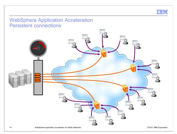
Persistent connections greatly reduce the TCP handshake overhead, but this situation is further optimized by maintaining connection pools at the closest point of presence to a local group of user agents. This further reduces the load on the origin server and has security benefits as denial of service attacks can be detected close to the originator and can be dropped or filtered well before the origin server.
