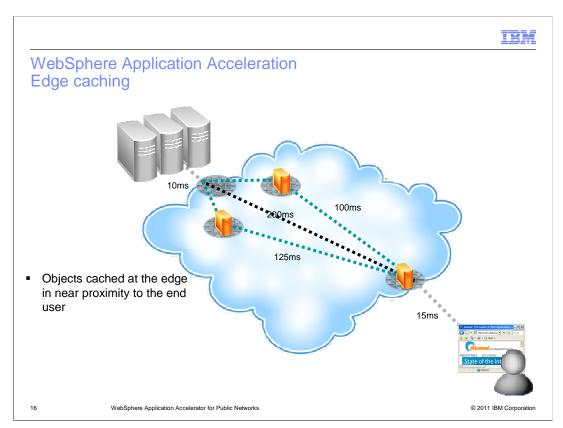
Edge Caching caches high frequency objects in near proximity to the consumer or end user. Caching reduces the number or round trips to the origin or dramatically reduces the quantity of data transmitted from the origin to the end user. When combining IBM WebSphere DataPower technology it is possible to enable the Akamai network to cache dynamic content, over and above the typically cached static content such as images and JavaScript.
