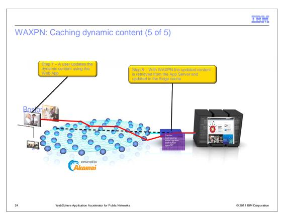
Dynamic content can be served from cache until it is modified through the web application. DataPower keeps track of HTTP PUT, DELETE and POST operations. Akamai EdgeServers check back regularly with DataPower to see if the dynamic content has been modified.... If not serving from cache continues. If so, the request is allowed to flow through DataPower to the application server to get the current version and the process starts again.
