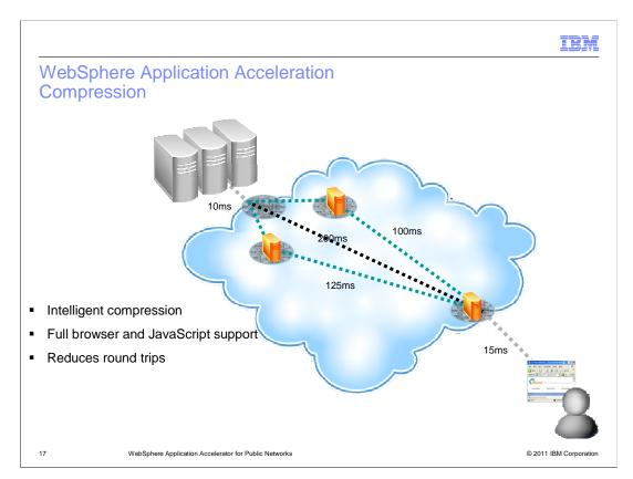
Intelligent Compression compresses content to reduce the size and therefore the latency required to transmit the objects across the Internet. A typical 100k byte page compresses down to 15k bytes. Intelligent compression ensures that already compressed objects are not double compressed and that compatibility is maintained regardless of user agent type or version.
