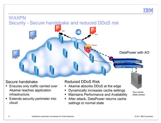
The WAXPN network fabric is designed to absorb DDoS
