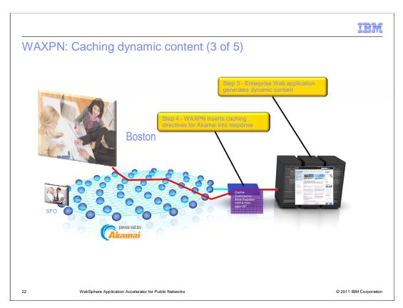
The response is generated by the backend application servers. The DataPower appliance adds special caching instructions to the response based on the policy specified.
