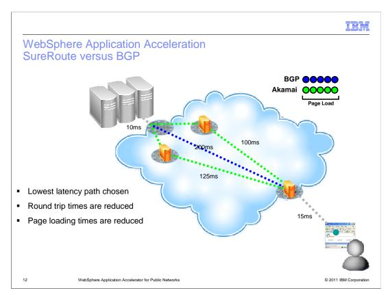
Sure Route verses B G P. Because the lowest latency path is chosen, the reduction in page rendering times is cumulative. Complex web applications require many round trips between the user agent and the origin server, and even the smallest improvements in latency, add up quickly to a user visible difference.
