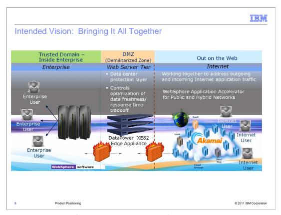
The graphic displays the full end-to-end use cases for the DataPower XE82 Edge appliance. The XE82 is deployed in the DMZ acting as a gateway for Web applications and Web services. The XE82 provides self balancing with failover, intelligent load distribution to backend application servers, acceleration, offload, authentication/authorization, governance and many other key features.
