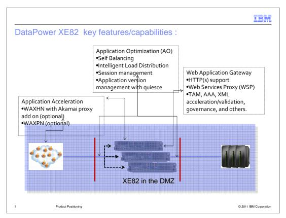
The DataPower XE82 appliance is generally deployed in the DMZ to accelerate and improve security for web applications and cloud services. Two or more XE82 appliances can be deployed for high availability and scalability. The standard Application Optimization functions provide self balancing to distribute incoming loads across the group of appliances with fail over. Other features include:
