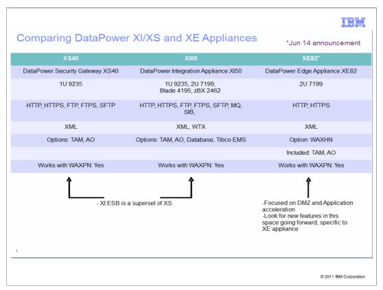
Comparing the DataPower XE82 edge appliance to the XS40 and XI50, the XE82:
