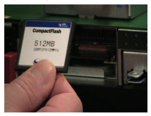
10. Align the new storage card (label-side up), and insert it into its socket until you hear it snap into place. Do not use excessive force to insert the storage card.
