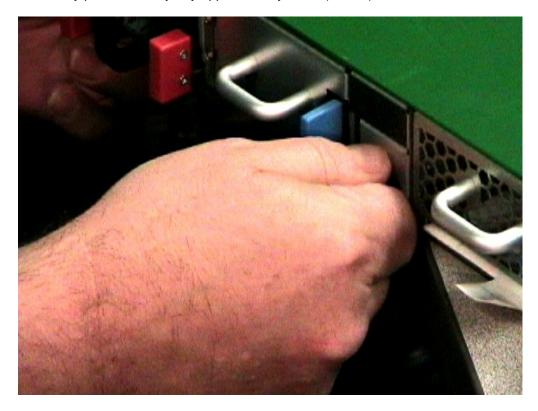
4. When the battery tray is fully extended, remove the battery from its cradle by pulling up on the clear polyester tab that covers the battery. Set the failed battery aside.
