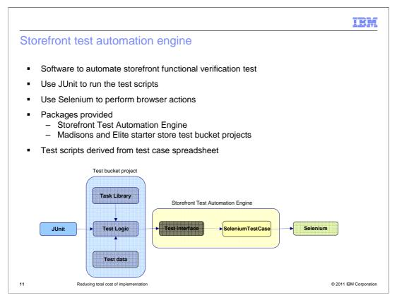
Storefront automation harness is provided to assist in automating functional verification testing. It consists of four key assets: JUnit, test bucket project, Storefront Test Automation Engine and Selenium.
