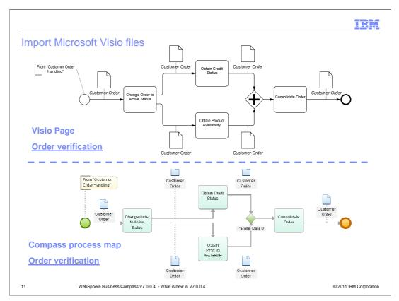
The screen capture at the top shows a Visio diagram and the screen capture at the bottom shows the corresponding compass process map that is created after uploading the Visio file.
