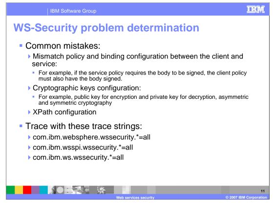
Common mistakes related to Web Service Security often deal with mismatching the policy configuration between the client and the service. When this occurs the client or service may not receive a message with the appropriate encryption or tokens that are expected. The trace strings to use for WS-Security are listed here for reference.
