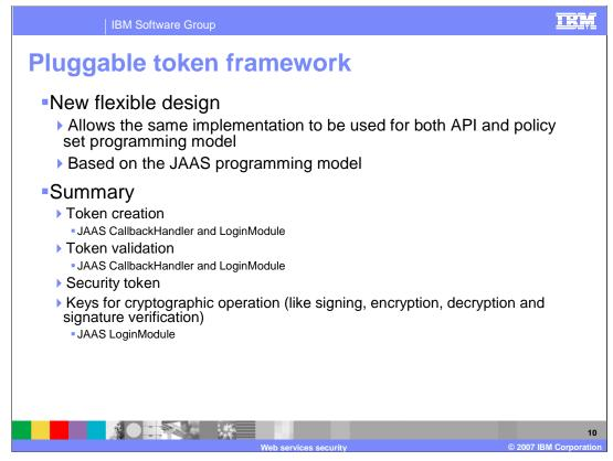
The token processing and pluggable token architecture in the Web Service Security runtime for IBM WebSphere Application Server V6.1 Feature Pack has been redesigned to reuse the same security token interface and JAAS Login Module from the Web Services Security APIs. The same implementation of token creation and validation can be used in both the WS-Security API and the WS-Security SPI in the Web service security runtime.
