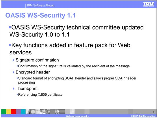
The OASIS WS-Security group has updated the specification to 1.1. The Feature Pack for Web Services adds support for several key functions from this specification, including; signature confirmation, the ability to encrypt SOAP headers, and the ability to add a thumbprint that references an X.509 certificate.
