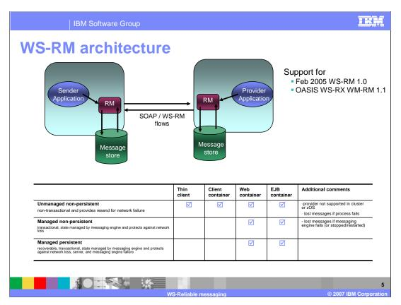
The architecture for WS-reliable messaging allows for SOAP messages to be placed in a message store on both the provider and sender applications. There are three levels of persistence available for WS-reliable messaging in the Feature Pack for Web Services; unmanaged non-persistent, managed non-persistent, and managed persistent. Each of these persistence levels has certain capabilities shown in the chart above, and explained further on the next slide.
