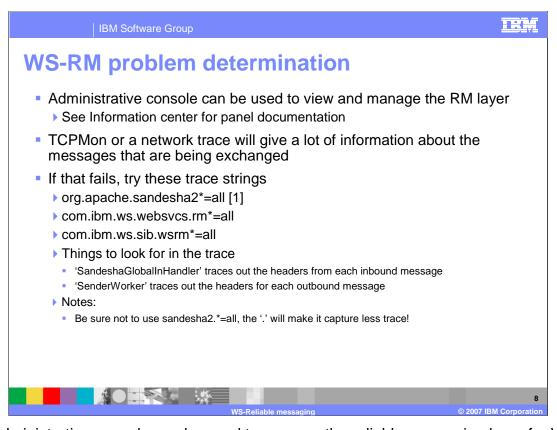
The administrative console can be used to manage the reliable messaging layer for Web services applications. Messages can be viewed and managed through various panels. Documentation can be found in the Information center for the Feature Pack for Web Services. A TCP monitor can be used to view the messages that are being exchanged over the network. Otherwise the above trace strings can be used to provide additional information specific to WS-reliable messaging problems.
