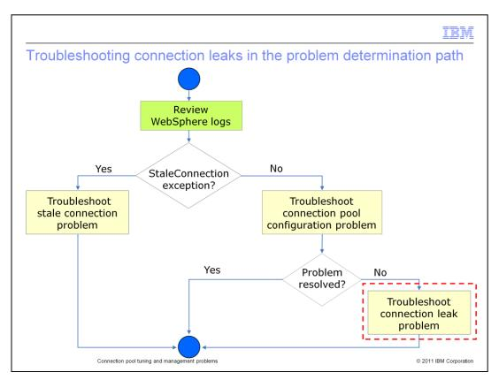
After you have ruled out the possibility of a stale connection and connection pool tuning problem, consider the possibility of a connection leak.
