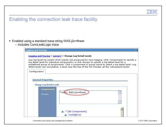
The connection leak trace facility is enabled through the AdminConsole.
