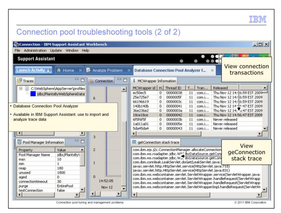
The IBM Database Connection Pool Analyzer tool employs a heuristic analysis engine to help you resolve problems related to Java Database Connectivity (JDBC) connection pools and find JDBC connection leaks.
