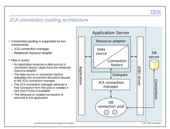
WebSphere Application Sever implements connection pooling by following the Java EE Connection Architecture version 1.5 specifications.
