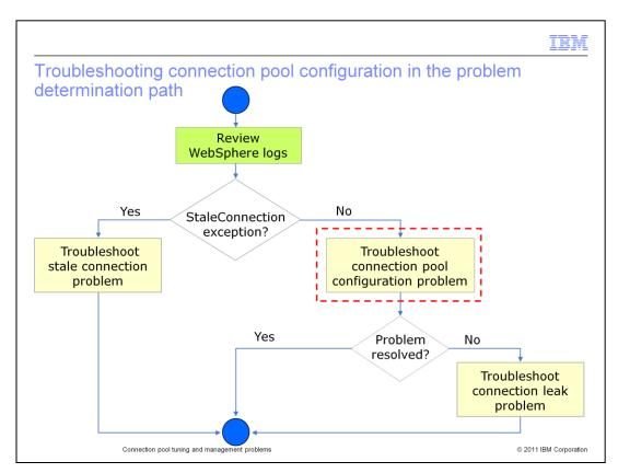
In the case where the symptom for a connection pool problem is not accompanied by a StaleConnectionException in the WebSphere logs, start your problem determination effort by looking at the connection pool configuration to rule out any performance tuning issues.
