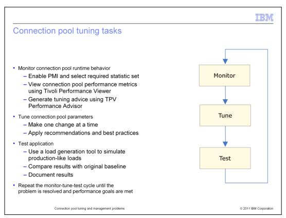
Performance tuning, in general, is an iterative and incremental process consisting of multiple Monitor-Tune-Test cycles. Having the right tools, including a load generation tool to simulate real-world users for load testing, is critical to ensure successful results.
