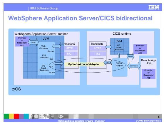
Above is a diagram demonstrating optimized local adapters between a WebSphere Application Server runtime and a CICS runtime. The CICS runtime, connecting to WebSphere Application Server uses supporting CICS communications called true, which is a task related user exit. CICS provides a set of APIs if you want to be a resource manager.
