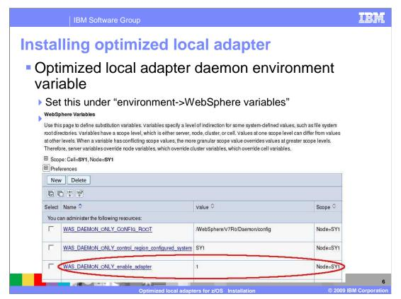
Above is a screen capture of the WebSphere Application Server environment variable WAS\_DAEMON\_ONLY\_enable\_adapter that needs to be set to 1 to enable the adapter support. Once set to 1 the Daemon will need to be recycled. If successful, in your Daemon log you will see enable\_adapters=1, the control and servant region will still indicate enable\_adapters=0, this is expected.
