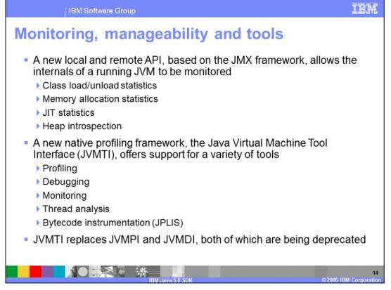
JDK 5.0 includes some manageability and tool enhancements. The JMX specification from J2EE 1.4 is now included in the standard J2SE specification for 5.0. These statistics gathering and investigative tools are now a part of the base JDK. The other major change is the deprecation of JVMPI and JVMDI which are being replaced with JVMTI, the Java Virtual Machine Tool Interface. This is a new profiling framework that supports a variety of debugging, monitoring, and code analysis tasks.
