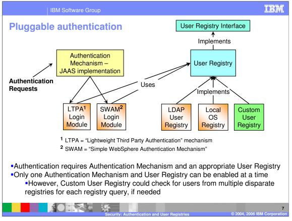
This slide shows the architecture of the Pluggable Authentication, where there are 2 Authentication mechanisms (LTPA and SWAM). Each one of them can use any one of the supported User registries (Local OS, LDAP or Custom Registry). Details of the Authentication mechanism and user registry are in the next few slides.
