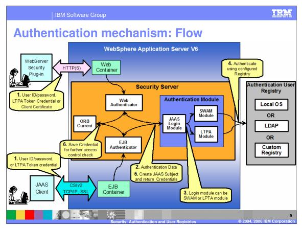
This picture shows a more detailed flow of the authentication process for both Web clients and EJB clients.
