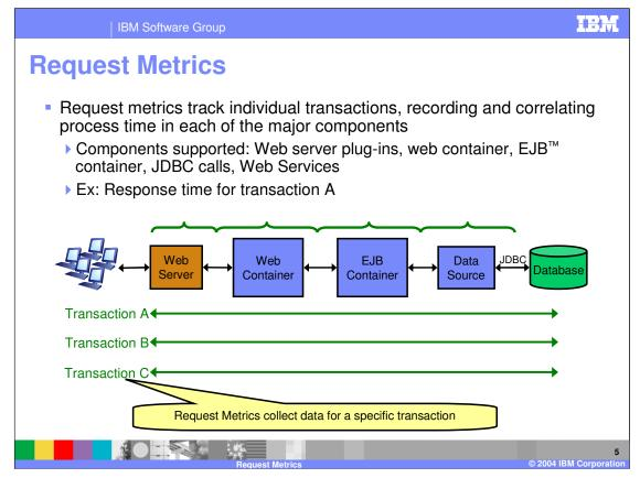
Request Metrics allow you to monitor transactions as they move through the different components in a WebSphere environment (HTTP server plug-in, Web/EJB container and database levels). Request monitoring can follow requests as they fan out across a WebSphere environment, monitoring them even as they cross process and host boundaries.
