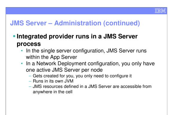
The integrated JMS Server itself is defined differently for Base and Network Deployment. In the base or single server configuration, JMS Server runs within the Application Server's JVM. In the Network Deployment edition, the JMS Server is started in its own JVM. There can only be one JMS Server defined on a given node.
