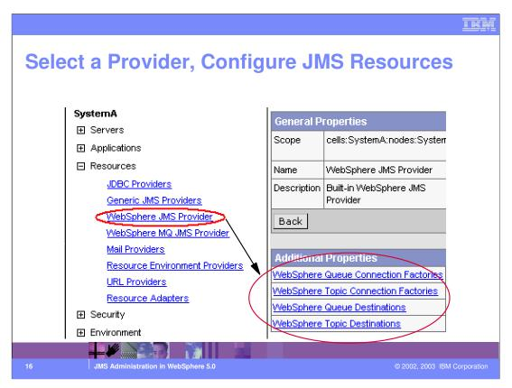
You can use the WebSphere administrative console to configure the internal WebSphere JMS provider or an MQSeries JMS provider. If you install another JMS provider, you need to configure that JMS provider by using the tools and information provided with the JMS provider. For each JMS provider, you can configure the properties of JMS resources.
