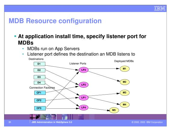
Once the JMS resources have been configured, deploy the MDB, specifying the ListenerPort, with which it is to be associated. Note that the listener port is in turn associated with the connection factory and the destination JNDI name.
