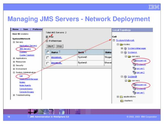
In an Network Deployment installation, the JMS Server is basically the Broker and additionally manages the QueueManager. It is a peer of the other servers in a given node, and it runs in its own JVM. There can only be one JMS Server defined on a given node.
