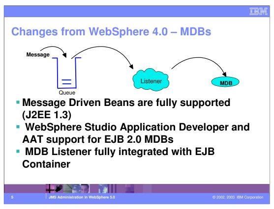
A Message-driven Bean is a stateless component that is invoked by the J2EE container (app server) as a result of the arrival of a JMS message at a particular JMS Destination (that is, a Queue or a Topic). You think of the MDB as being "triggered" by the arrival of a message. The Listener component is the part of the Application
