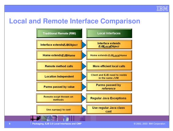
This chart summarizes the differences between local and remote interfaces. It's important to notice that, while an EJB may offer both local and remote interfaces, the choice of using local or remote in the EJB client is NOT transparent. The client code will clearly reflect which interface is going to be used.
