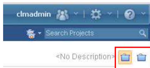
Figure 10.: The left icon opens the current project. The right icon deletes the baseline.
