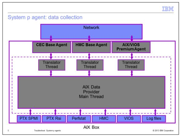
The Tivoli Monitoring System p agents use several mechanisms to collect data, depending on the attribute group. The most important ones are SPMI (System Performance Measurement Interface) and RSI (Remote Statistics Interface). These mechanisms are also the interfaces that are the most error-prone, and often cause a lack of data in the Tivoli Enterprise Portal.
