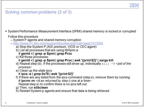
If you encounter a shared memory lock or corruption, follow the procedure described on the slide. You must apply it on the local LPAR when the agent has trouble collecting data from its own LPAR. Or you can apply it if the agent has difficulties in collecting correct data from a remote monitored LPAR.
