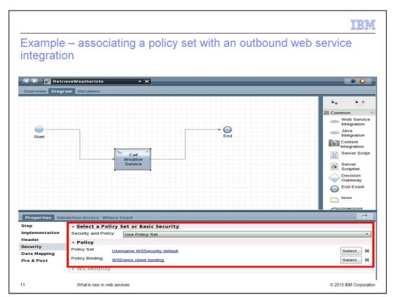
This slide shows an example of how to associate a policy set and binding directly with an outbound web service integration, without the use of a web service server configuration. For the Security and Policy field, you choose "Use Policy Set" and then, in the Policy section, you select your desired policy set and binding.
