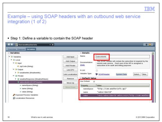
This example shows you how to use a SOAP header within an outbound web service integration. Suppose that your outbound web service integration needs to invoke a fee-based web service endpoint, which requires its customers to include a "subscription identifier" along with the request message for billing purposes.
