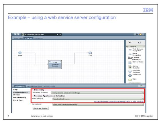
This example shows how to use a web service server configuration when defining an outbound web service integration. Within Process Designer, you can choose "From process application settings" for the "Discovery Scheme" option, then select the required server configuration.
