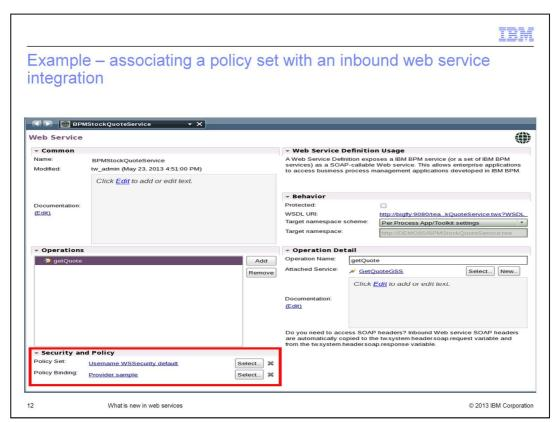
This slide shows how to associate a policy set and binding with an inbound web service integration. In this example, the web service endpoint is being protected with username token security.
