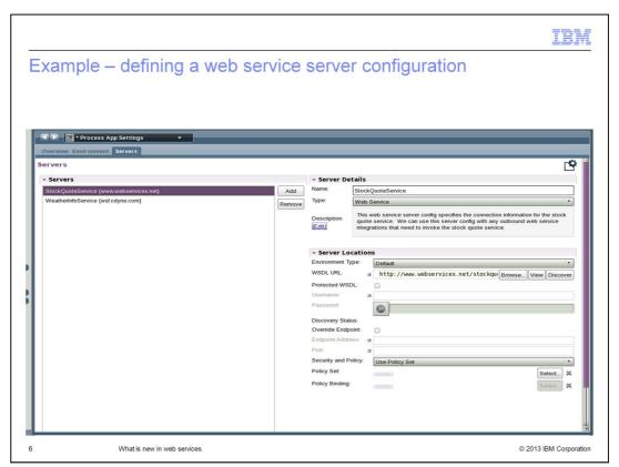
On this slide is an example of a web service server configuration that is defined within the Process App Settings view of IBM Process Designer. In this example, the server configuration contains the connection details of a provider named StockQuoteService.
