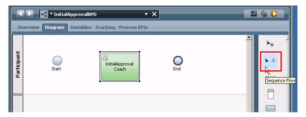
\_\_ k. Click the right side of the Start icon to start the wire, then move the pointer to the left side of the InitialApprovalCoach and click to complete the wire, connecting the two.
