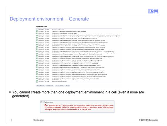
When the configuration completes, you can examine the configuration files to view the changes. Either save the changes to the master configuration or discard them.
