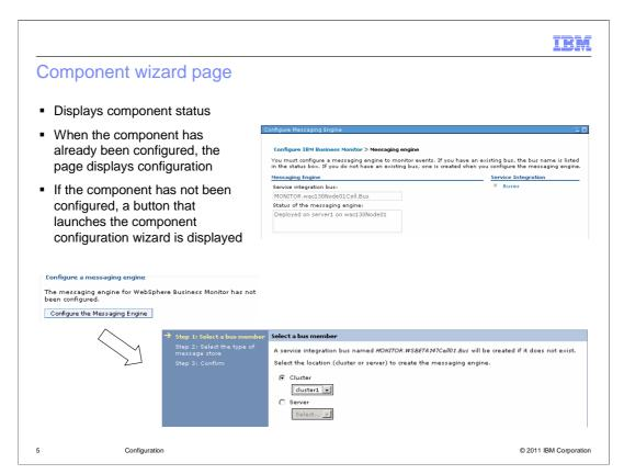
This is a sample of the messaging engine component configuration page. It shows the current component status if the component has been configured previously. If the component is not configured, then you will also see a button that will launch the configuration wizard.
