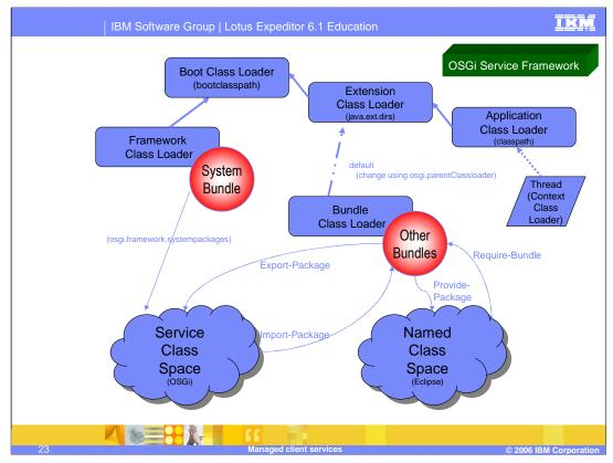
Class loading functions differently than a typical Java application because the client platform is built on the OSGi Service Framework. Since the mechanics for supporting plug-ins are implemented by using the OSGi Service Framework, a plug-in is the same as an OSGi bundle for the purpose of this explanation. The bundle and its associated classes specify and implement the process for Java class loading, prerequisite management, and the bundle's life cycle.
