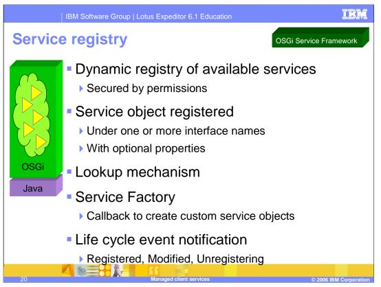
In the OSGi environment, bundles are built around a set of co-operating services that are available from a shared service registry. The service interface defines the OSGi service, which is implemented as a service object.
