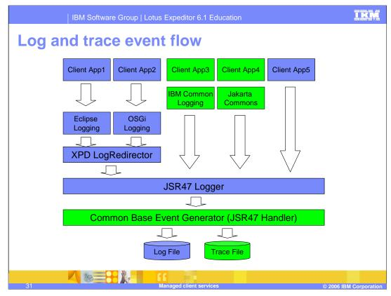
This diagram gives a high-level overview of the logging system in Expeditor 6.1. Applications may choose to log using many different mechanisms, including OSGi logging, Eclipse logging, IBM Common logging, and Apache logging, however they all consolidated at the JSR47 logger level so that all log messages are logged to one file.
