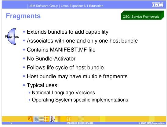
A component may not always provide a complete implementation. In some cases, *fragments* may be used to complete or extend a component. For example, the primary component may provide an implementation that contains translatable text in a default language. Fragments are then used to provide translations for additional languages.
