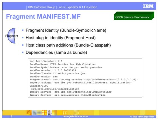
Fragments contain either a fragment.xml (similar to a plugin.xml), or a MANIFEST.MF, or both. A fragment is associated with, or dependent upon, a specific primary component, but still maintains a unique identity. Querying a list of components will also return fragments, so that these fragments can be individually started and stopped.
