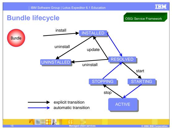
The framework manages the life cycle of bundles. As you install and run a bundle, it goes through various states. The possible states of a bundle are:
