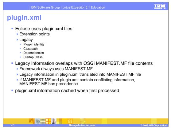
Each bundle must contain either a manifest file or a plugin.xml file. The bundle's manifest file contains data that the framework needs to correctly install and activate the bundle. Legacy Eclipse bundles can provide some manifest information in their plugin.xml files, but META-INF/MANIFEST.MF files are the recommended files for Manifest information. Note that a plugin.xml may contain similar information, however, a plugin.xml also contains extensions and extension points.
