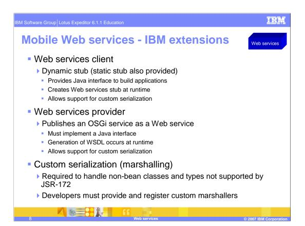
A dynamic stub allows you to decide to use Web services at runtime rather than build time, that is, dynamic stub allows Web services to be configured and deployed in the field without involving a build team. A dynamic stub also allows a Web services client to create and use custom marshallers for WSDL types that are non-bean classes or incompatible with JSR-172.
