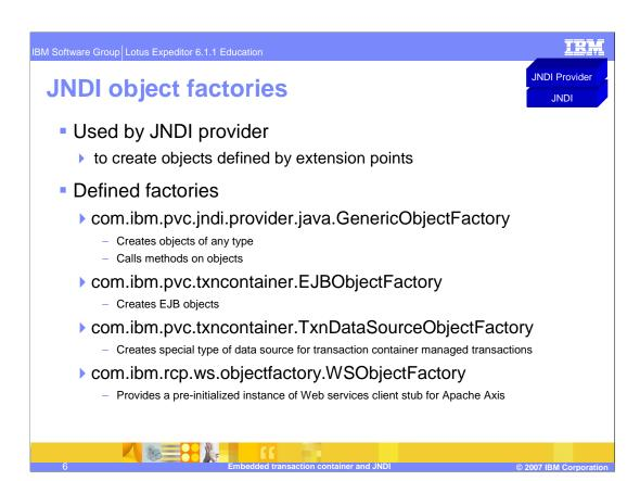
The JNDI object factories are used by JNDI provider to create objects defined using extension points. The defined factories are listed on this slide and the next slide.
