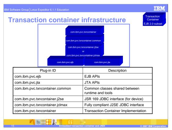
This slide shows the Transaction Container infrastructure on the client platform, including the plug-ins (components) installed with the client platform and a description of each of these plug-ins.
