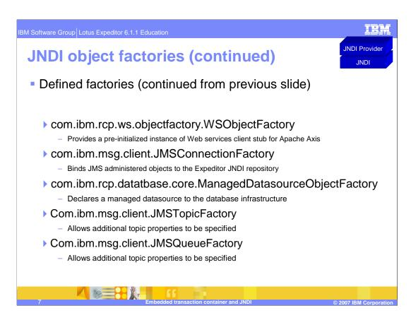
The JNDI object factories are used by JNDI provider to create objects defined using extension points. The defined factories listed on this slide are continued from those listed on the previous slide.
