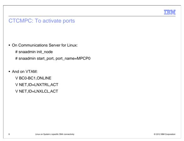
Here are the commands for activating ports on Communications Server for Linux and on VTAM.
