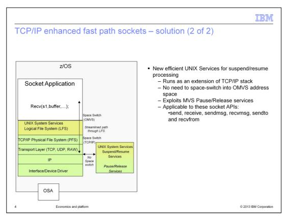
The enhanced fast path sockets support exploits the new efficient UNIX Services suspend and resume processing. These services run as an extension of TCP/IP and so the space switching into OMVS address space is not done.
