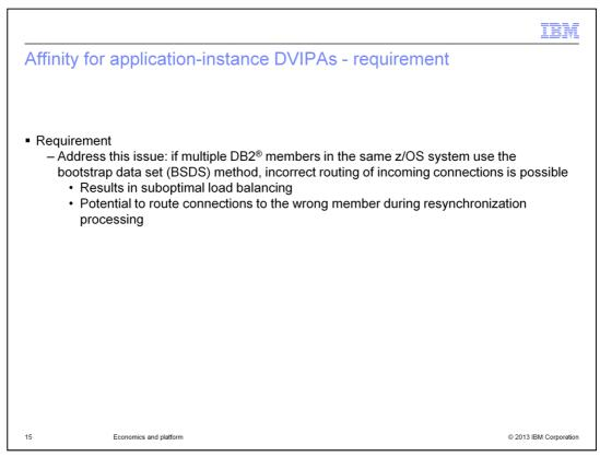
The DB2 bootstrap data set approach can result in incorrect behavior if more than one DB2 application is active on the same stack. Because each server uses inaddr\_any and the distributed dynamic virtual IP address port, there is no specific association of a server to an application-instance dynamic virtual IP address.
