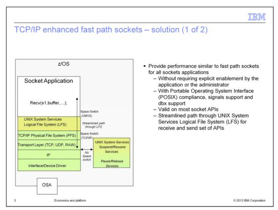
Here you see the processing that occurs for the enhanced fast path sockets support in V2R1. It does not have to be enabled and it is available to all the socket APIs, with the exception of the Pascal API. It performs better than the existing fast path sockets support.
