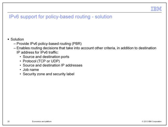
IPv6 policy-based routing enables the TCP/IP stack to make IPv6 routing decisions that take into account criteria other than just the destination IP address. The additional criteria can include job name, source port, destination port, protocol type, source IP address, NetAccess security zone, and security label. With policy-based routing, you can define a policy that selects the network to be used for outbound traffic, based on the application that originated the traffic.
