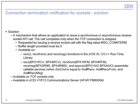
z/OS Communications Server provides a mechanism that allows an application to issue either a synchronous or asynchronous receive socket API call that completes only when a TCP connection is stopped.
