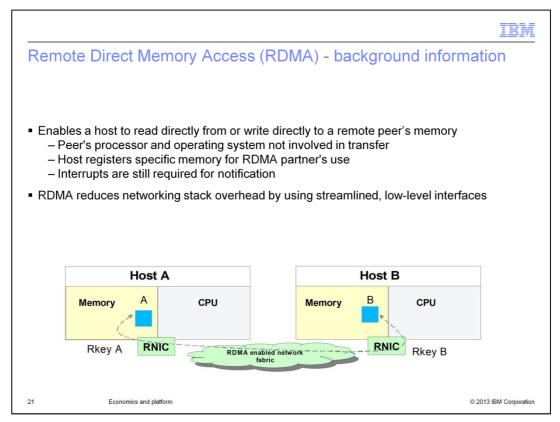
Remote Direct Memory Access allows a host to access memory on a remote peer that is connected to the same Remote Direct Memory Access-capable Ethernet fabric. Remote Direct Memory Access protocols allow a host to read from or write into memory that the peer has allocated specifically for use by that host.
