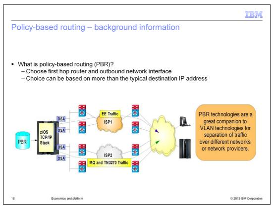
Policy-based routing allows IP routing to use additional route selectors. It is made possible through the use of multiple route tables. In addition to the main route table, the TCP/IP stack can have multiple policy-based route tables. Policy-based route tables have many of the same characteristics as the main route table. They can contain both static and dynamic routes and the static routes can be configured as both replaceable and non-replaceable.
