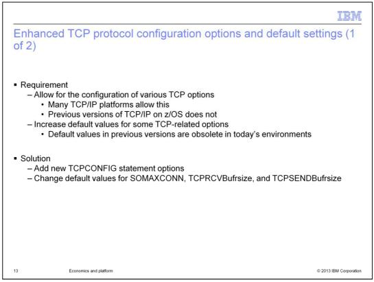
Many TCP/IP platforms allow for the configuration of various TCP options. For example, it is possible to specify how long connections remain in the TIMEWAIT state and the amount of time a TCP packet is retransmitted before aborting the connection. It is also possible to specify the number of times a TCP packet is retransmitted, the maximum number of keepalive packet probes sent, and whether Nagle's algorithm is globally enabled.
