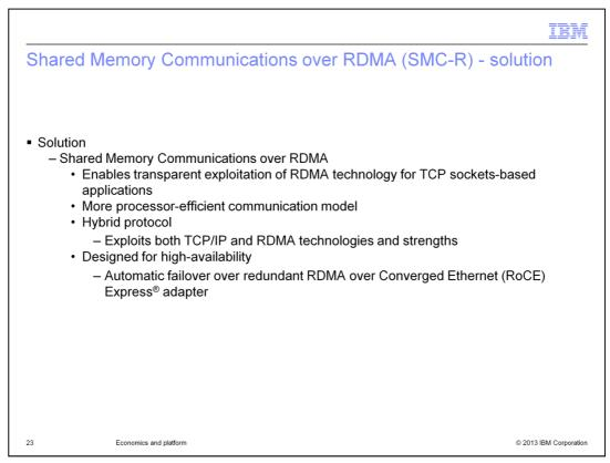
z/OS V2R1 Communications Server exploits RDMA technology by using Shared Memory Communications over RDMA protocols. These protocols provide a transparent socket-based exploitation model for RDMA, allowing existing TCP applications to benefit without change.
