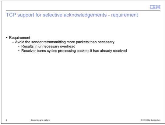
In previous releases, the TCP retransmit and acknowledgement logic is structured such that, when an out-of-order data packet arrives, the receiver responds with a duplicate acknowledgement. This signals to the sender that out-of-order data has been received and a packet has possibly been lost. When the sender receives three duplicate acknowledgements, it assumes that data has been lost in the network and resends the missing packet and all the packets that were sent after the missing packet.
