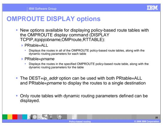
A new option has been added to the OMPROUTE DISPLAY RTTABLE command. The option is PRtable and it is used to indicate that OMPROUTE policy-based route tables are to be displayed. The values that can be specified on the PRtable option are ALL or the name of a policy-based route table. Use ALL to request the display of all OMPROUTE policy-based route tables. Use the name of a policy-based route table to display only that table.
