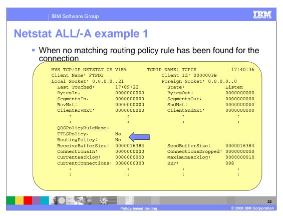
This example shows a connection for which a matching routing policy rule has not been found. Note that the RoutingTableName and RoutingRuleName fields are not displayed.
