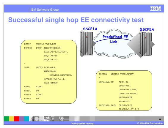
This is a sample of a single hop predefined Enterprise Extender (EE) link. This example illustrates a case where connectivity being tested between two EE endpoints is successful.
