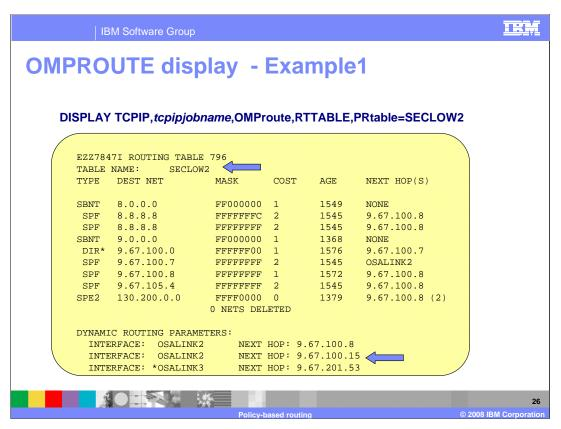
In this example, the PRtable=*prname* option has been used to display a particular policy-based route table. The *prname* value of SECLOW2 results in only that route table being displayed.
