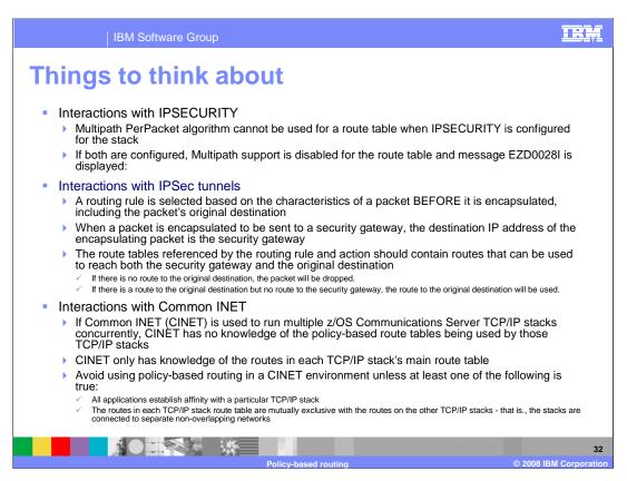
As with the main route table, the Multipath PerPacket algorithm cannot be used with a policy-based route table when IPSECURITY is configured for the stack. If these two are configured together, the Multipath function will be disabled.
