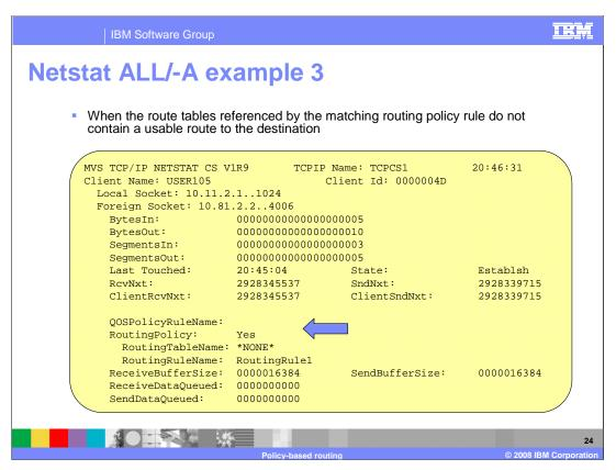
This example shows a connection for which a matching routing policy rule has been found. However, a search of all of the associated route tables has failed to find a usable route to the destination. When this is the case, the RoutingTableName is displayed as \*NONE\*.
