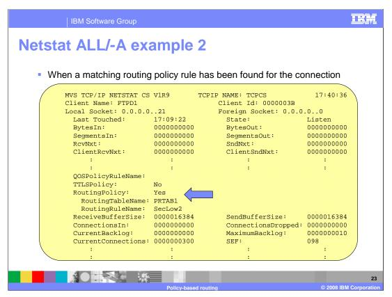
This example shows a connection for which a matching routing policy rule has been found. The RoutingTableName and RoutingRuleName fields are now displayed, showing the route table and routing policy rule being used.
