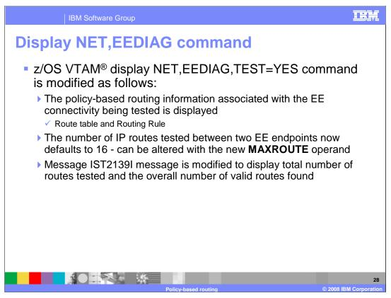
The Display EEDIAG, TEST=YES command, or Enterprise Extender (EE) connectivity test command, is useful in debugging various network problems and was introduced in z/OS V1R8 Communications Server. This command can be used to test an existing Enterprise Extender connection, or it can be used to assist in diagnosing why an EE connection cannot be established.
