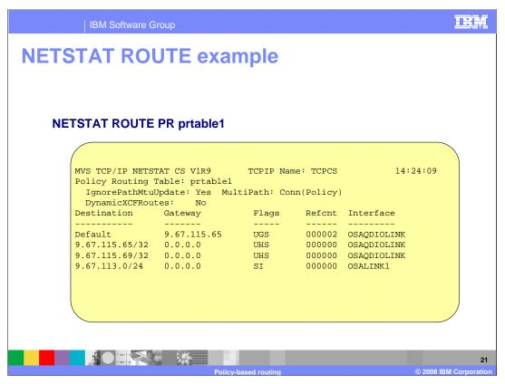
This example uses the PR modifier with the name of a policy-based route table. The resulting report includes the name of the route table, the three table-specific configuration values (IgnorePathMtuUpdate, MultiPath, and DynamicXCFRoutes), and the routes contained in the route table.
