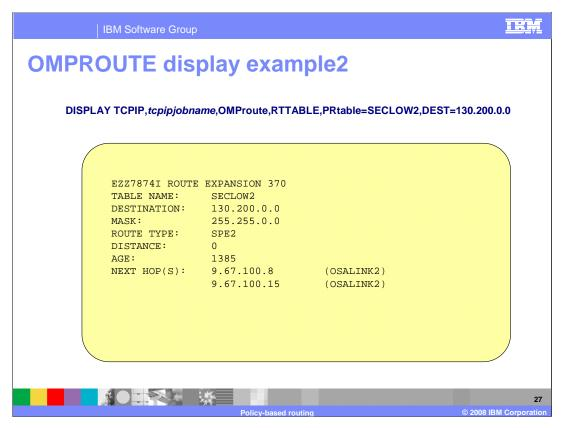
In this example, the DEST=*ip\_addr* option has been used in order to display the multiple next hops to the 130.200.0.0 network that appear in policy-based route table SECLOW2.
