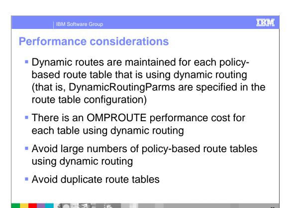
Each policy-based route table that is configured for dynamic routing adds additional processing to OMPROUTE. Duplicate route tables should be avoided and this is ensured if the Configuration Assistant is used to create your policy agent flat-files. In addition, you should avoid having large numbers of policy-based route tables that use dynamic routing.
