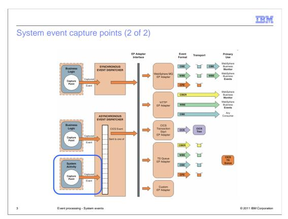
This diagram shows a high level view of event processing in CICS TS V4.2.
