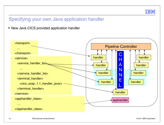
To incorporate the use of your own customized Java application handler, specify it in the pipeline configuration file in the <apphandler\_class> XML element.
