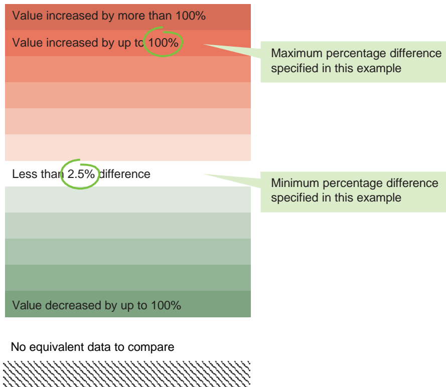
Figure 18. CICS PA Compare Before-After Excel add-in: sample comparison: how minimum and maximum percentage differences affect color highlighting
