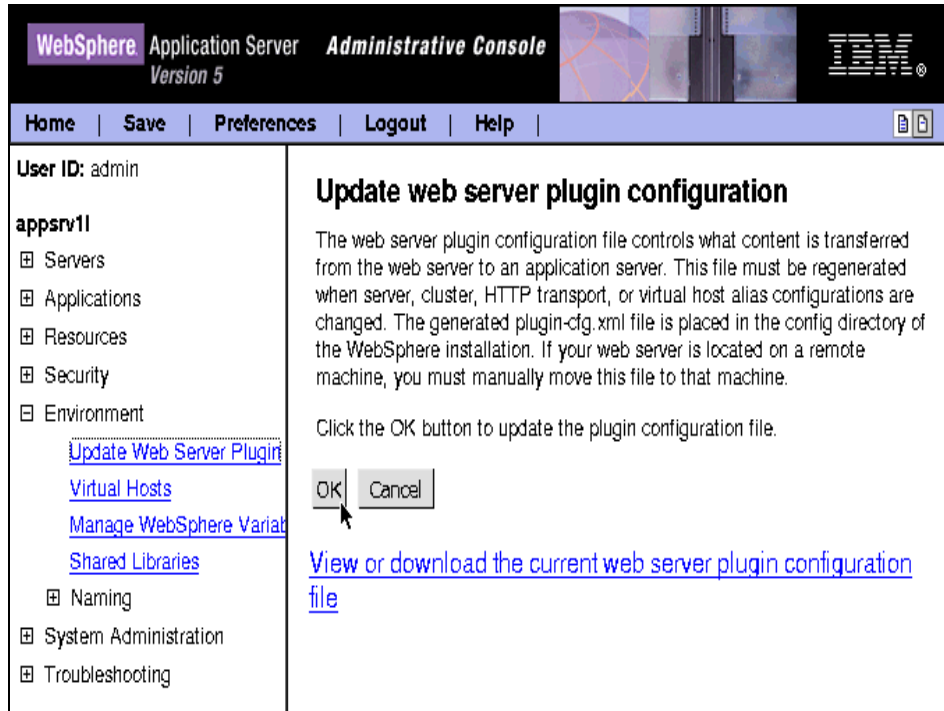
Figure 5-11 Regenerating the Web server plug-in configuration from the console
