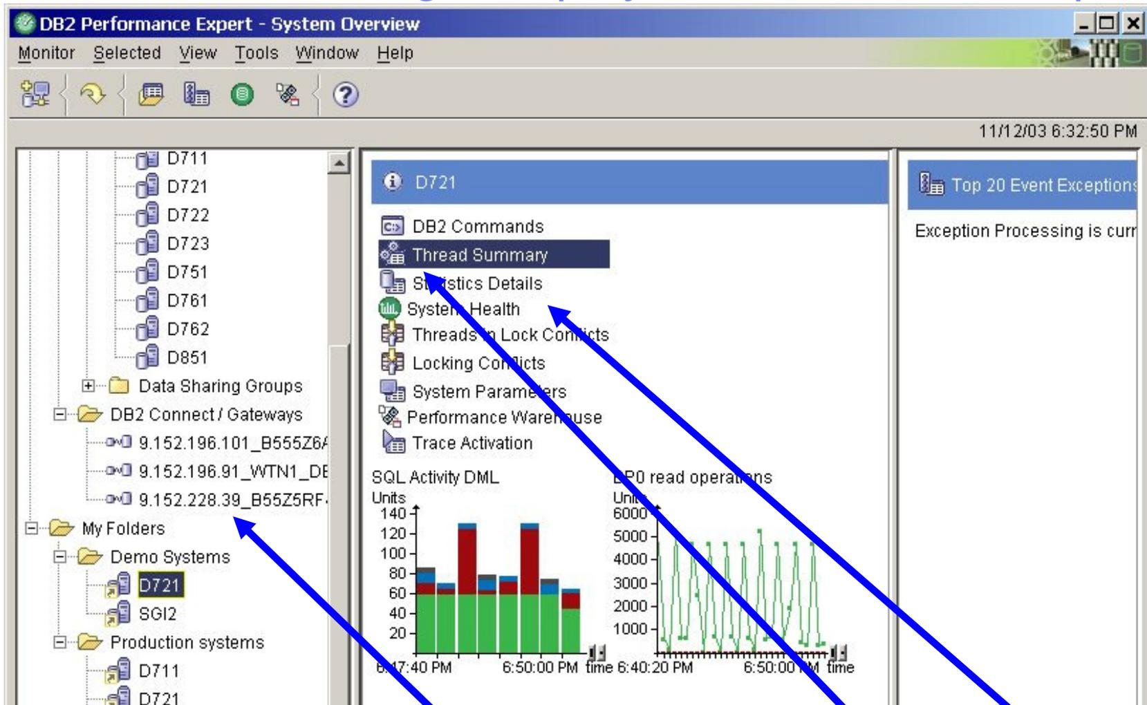
**Performance data from DB2 Connect can be shown from different perspectives: By monitoring the DB2 Connect itself or drilling down into thread and database statistics.**
