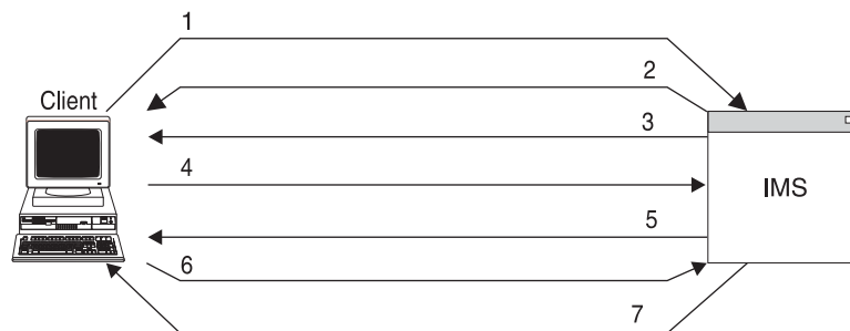
Figure 19. Flow of Resynchronization (Nondeferred)
